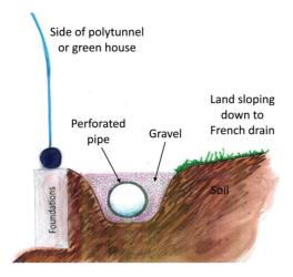
French drains capture water from the surrounding soil (not just the area immediately above). In other words, moisture moves sideways through soil into the drain.
