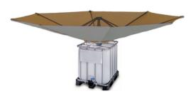
Another option is using a raised sheet to direct rainwater into a container. The challenge is protecting the sheet from strong winds which can exert considerable forces. Using an Intermediate Bulk Container (IBC) for water storage and keeping it partly filled can provide a secure base for the sheet.
